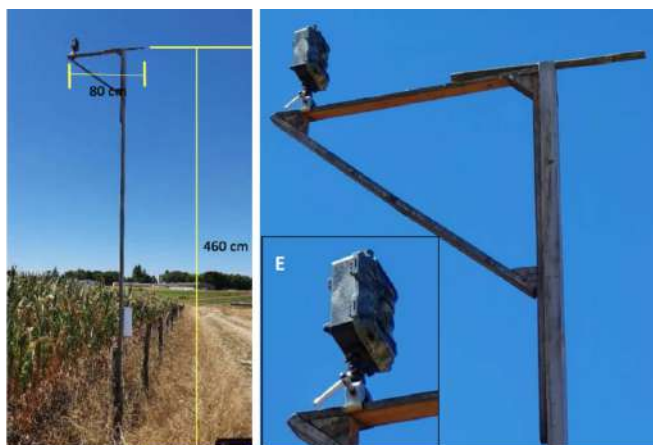
Figure 3.4. Setting and dimension of perches (on a fencepost), details of camera position, and camera clamped on wooden support. (From Beltramo & Goudet, 2025)
